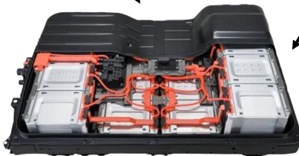
Li-ion NMC battery
