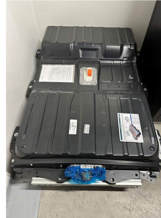
A photo of a Nissan LEAF battery from the L2EP lab
