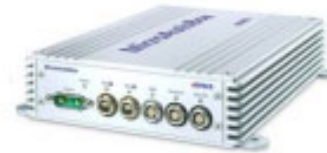
Real time computer can be connected to the CAR communication port (OBD)
