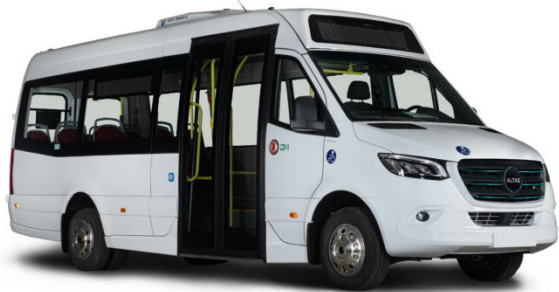
ALTAS interurban mini bus (5800kg / 20 seats / e-drive 160 kW / Li-Ion NMC Bat. 115 kWh) https://www.atlasautobus.com
